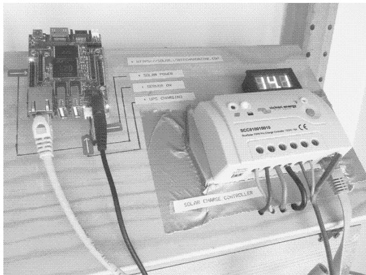
Image: The server and the solar charge controller.
